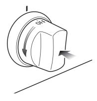
The maximum aperture position permits rapid boiling of liquids, whereas the minimum aperture position allows simmer warming of food or maintaining boiling conditions of liquids.
